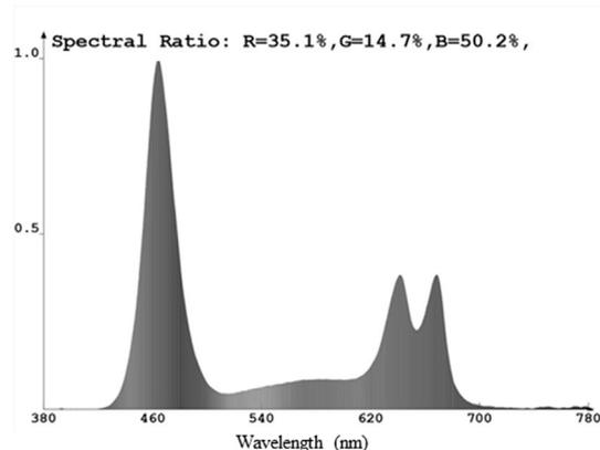
Fig. 1. A graph of the light spectrum produced by the light-emitting diode (LED) systems used in this study (Adapted from the product information sheet provided by the manufacturer: Shenzhen Bailuo Technology Co., Ltd., Guangdong, China).
